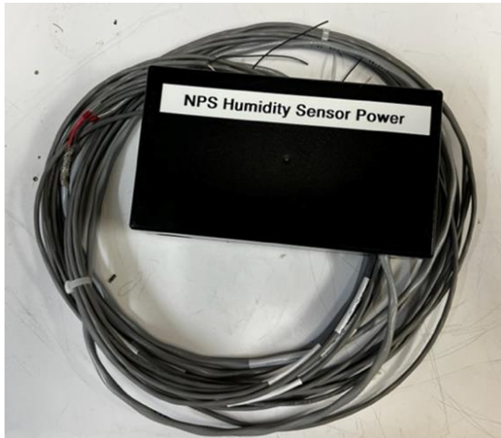
NPS eight-channel humidity sensor power distribution box
